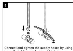
Connect and tighten the supply hoses by using two adjustable wrenches (avoid twisting or kinking).
